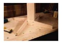
The feet are attached to the column with flat-head screws. Watch the screw alignment or you'll drill into another screw.
