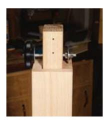
Some simple hardware from your local home center store allows you to lock the post solidly, but quickly loosen the post and readjust for any height. The hardware is shown at right, resting on top of the column before being attached through the holes.
